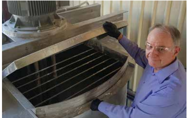
Senior 4Farmers Chemist, Dr Roger Franklin, with the new shear mixer that will ensure production of high quality suspension concentrates with finer particle size.
